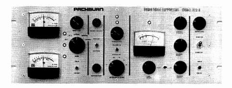
Three processors for reduction of transient and steady-state noises
